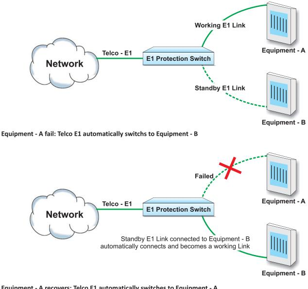
Equipment - A recovers: Telco E1 automatically switches to Equipment - A
