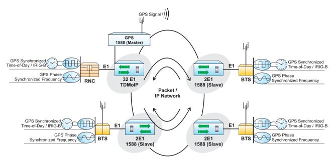
TDM over IP/Ethernet: Using IEEE 1588v2\* to distribute E1s, ToD (Time-Of-Day) and Frequency Synchronization over a Complex Ring and Spoke Optical Fiber Networks
