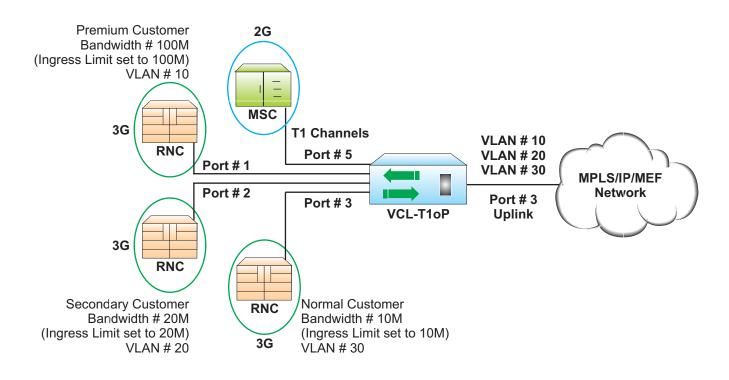
**Notes:** Port based Ingress Ethernet Rate Limiting allows the service provider to assigned the bandwidth as per customer requirements and separating their traffic by assigning 802.1Q based VLANs.
