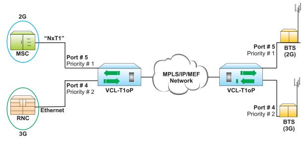
**Notes:** Port based Priority feature allows the user to assign priority to the 2G and 3G traffic ports, so that traffic can be regulated according to the port on which that service is connected.
