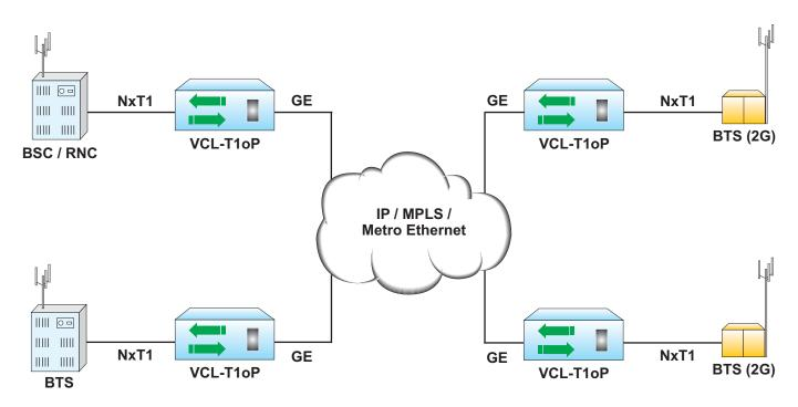
Note: Application illustrates link protection using Spanning Tree Protocol between all nodes.
