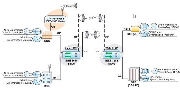
TDM over IP for 2G/3G/LTE in a redundant Wireless Network (1+1 Link Redundancy) with IEEE 1588 v2\* Synchronous Ethernet
