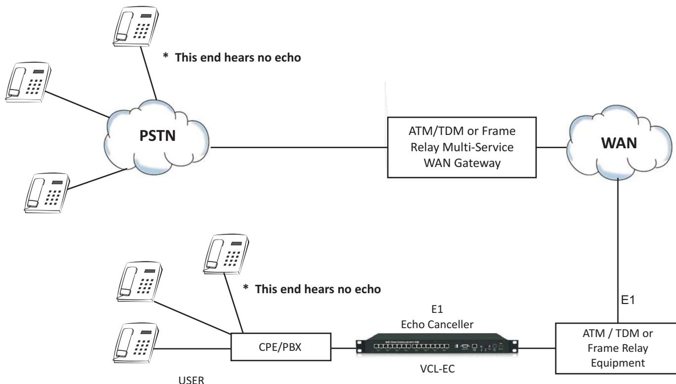
To cancel the echoes at both ends of the network with one 128ms. bidirectional Echo Cancellor with user programable Echo Tail Displacement (Echo Tail Off-set) Features
