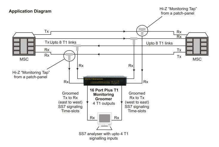
Note: The T1 link is "tapped" through a Hi-Z "Tapping" Port of a DDF Patch Panel.
